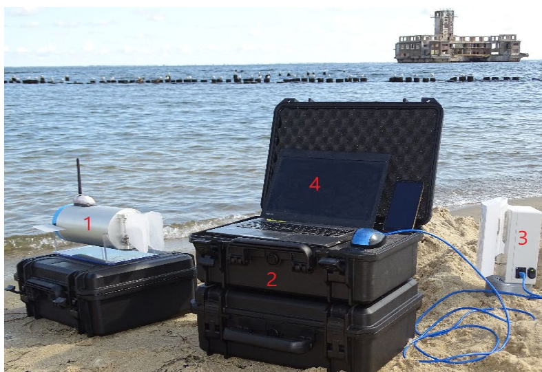
1 – biomimetic unmanned underwater vehicle; 2 – transport case; 3 – transceiver unit; 4 – mission planning and monitoring computer.
