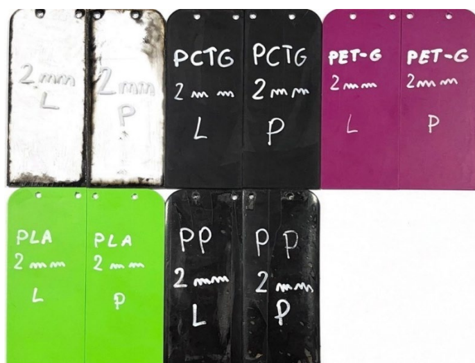
Figure 4. Fins fabricated from materials with diverse mechanical and technological properties
