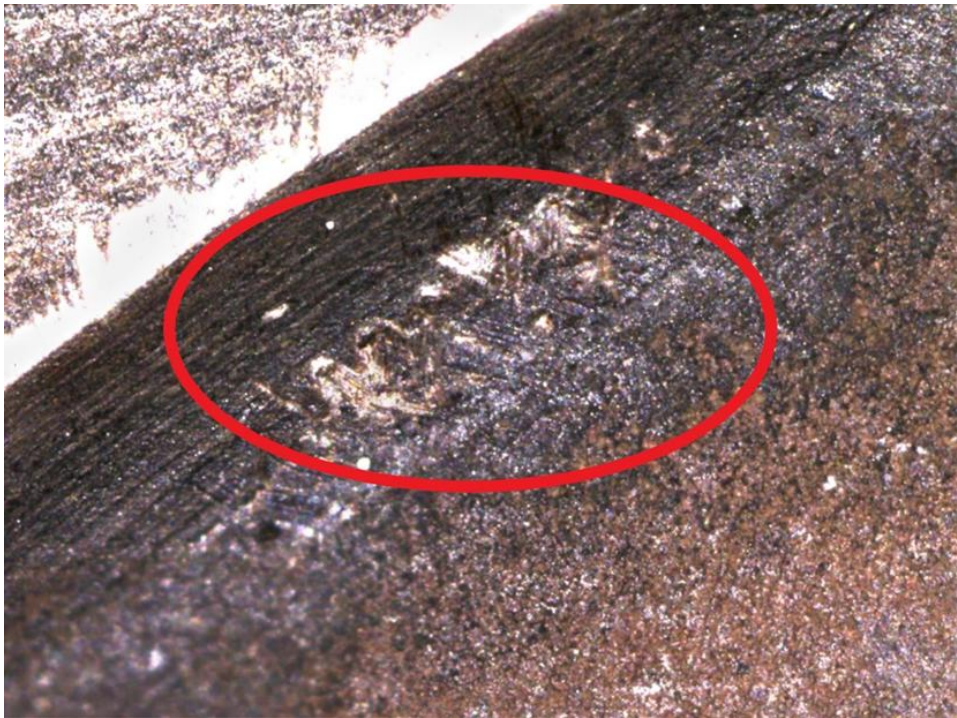
Fig. 4. Traces of piston–exhaust valve contact
