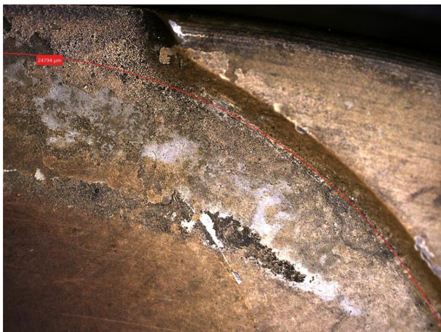
Fig. 6. Imprints with a diameter close to that of the valve head
