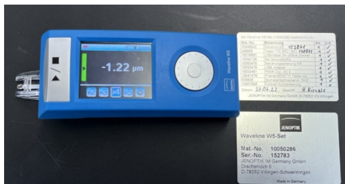
Fig. 4. Waveline W5-Set profilometer
