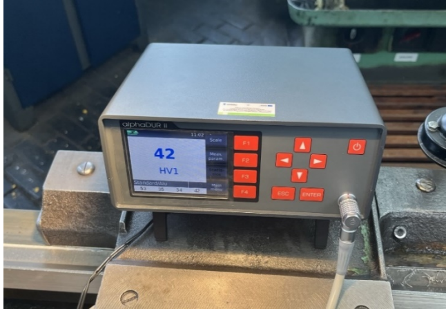
Fig. 5. AlphaDUR II ultrasonic hardness tester
