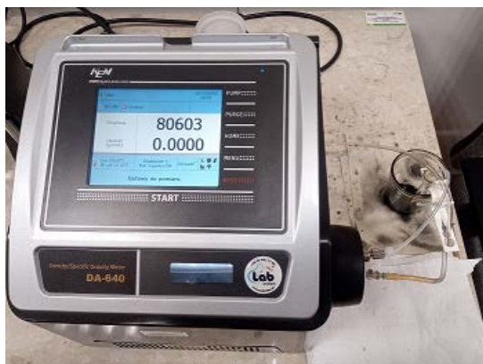
Fig. 4. Oscillating density meter DA640 used in oil tests
